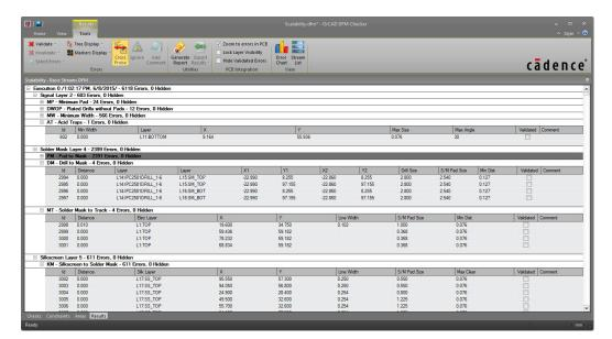
Figure 1: Use OrCAD DFM's charting feature to identify design issues with the potential to result in low manufacturing and assembly yields or costly scrap.
